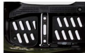
Full floorboards with drain holes
